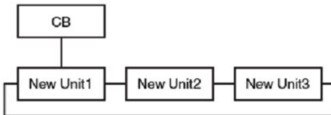
FIGURE 28 Case 1: Ring of Potential PEs with One Direct Connection to the CB
