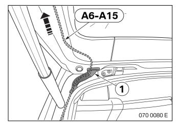
Thread connecting points **A6** to **A15** through rubber grommet (1) in tailgate, left side.
