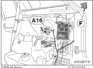
Route connecting point **A16**, RTGN, to the fuse carrier on the right of the luggage compartment.
