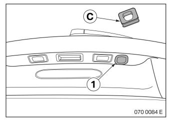
Remove protective cap (1) from tailgate and insert rubber seal  ${\bf C}$  in aperture.
