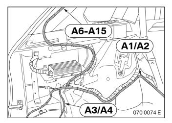
Route connecting point of cable kit rear-view camera **A** as follows:
