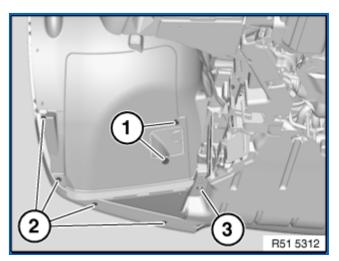
Release expander rivets (1) and screws (2, 3).
