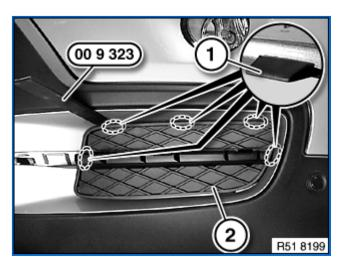
Push down latch mechanisms (1) with special tool <u>00 9 323</u> and remove ornamental grille (2) towards front.
