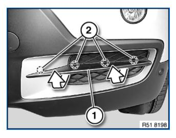
Detach side gill (1) in direction of arrow from latch mechanisms (2).
