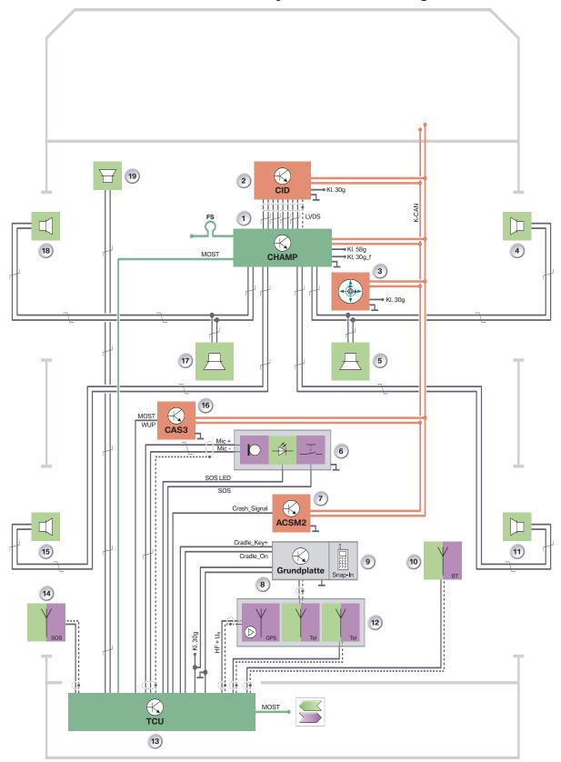
TCU with "Professional" Radio System Circuit Diagram
