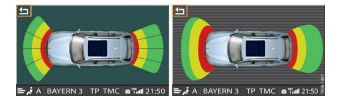
The park distance control is shown in the central information display when visual distance signalling and park distance control have been activated.
