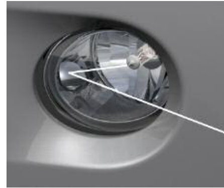
The turn-off light function is integrated in the fog light. This function is active only in position "A" of the light switch.
