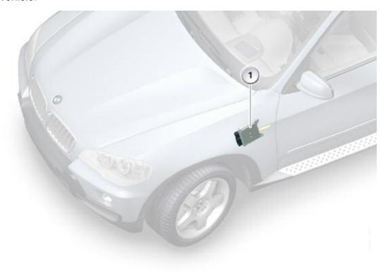
The AS control unit is integrated into the vehicle electrical system by the PT-CAN and the F-CAN. The AS control unit calculates the control signals for the AS actuating unit from various input signals.
