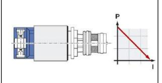
Electronic pressure control valves 3, 7: Blue cap, rising characteristic
