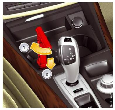
In the event of the system voltage failing, first release the electro-mechanical parking brake (EMF) as the handle remains in the emergency release.
