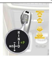
A drive range or neutral "N" can be engaged from "P" only with the unlock button pressed and the service brake depressed.
