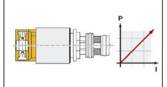
Electronic pressure control valves 1, 2: Orange cap, rising characteristic Technical data:
